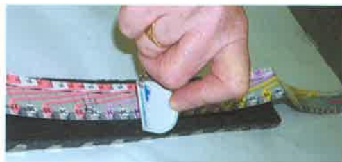
Place the measured tape along Grafitec and cut it.
